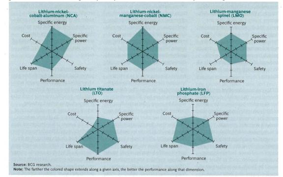
Figure 21. Boston Consulting Group Comparison of Lithium-Ion Battery Technologies
